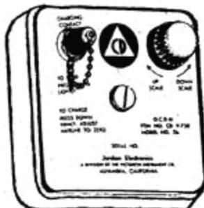
A Dosimeter Charger is used to charge or "ZERO" the Dosimeter.
